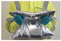
2. To start the mixing process hold the bag as shown by the hardener (small) compartment.
