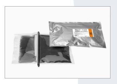
PC5581 is a cold curing 2-component polyurethane resin specially designed for cablejoints up to 1 kV. PC5581 has good anti corrosionproperties and shows a good adhesion to metals, ceramics, and many different plastics, and can be utilized on all plastic- and paper isolated cabletypes.
