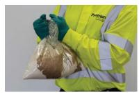
4. Squeeze the liquid through the membrane seal and onto the powder.
