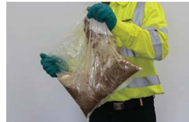
6. Before mixing rotate and shake at the corners to free the powder.
