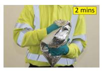
5. Tumble and knead the bag to mix the two liquids for up to two minutes.
