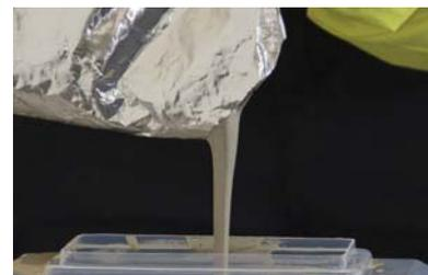
8. Pour pouch contents into the joint shell.
