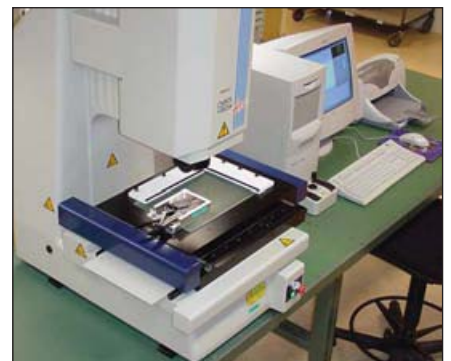
Production station for measuring crimp die nest heights.
