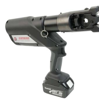
**PVL1300** is a battery powered crimp tool with 13 tons force. Uses the same crimp accessories as the other products in the 1300-System.
