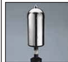
ERITECH ® INTERCEPTOR INTMKIV-SS (702089) 2 kg Air terminal for smaller protection areas or structures <20 m tall.
